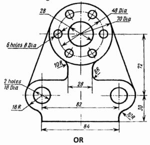
Q.1(B) Draw the figure shown below using Auto CAD commands and dimension it.
