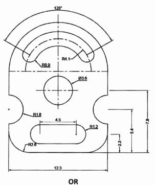
Q.1(B) Draw the figure shown below using Auto CAD commands and dimension it.
