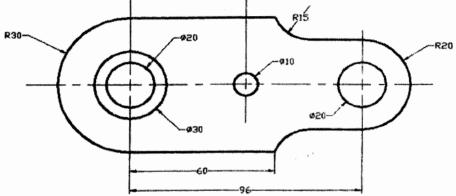
Draw the figure shown above using Auto CAD commands and dimension it.
